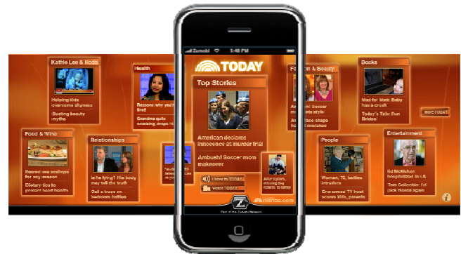
Figure 2: Recent ZUI: Zumobi's ZoomCanvas zooms in from the entire canvas on startup. Dragging left/right pans, and tapping on a region zooms in for interaction with the detailed content (2009) [54].
